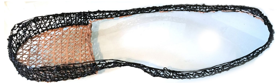
The resulting sole, with a 'wood effect' filament on the heel.
